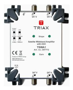
The amplifier has selectable inputs between Wideband LNB (290 - 2400 MHz) and Universal LNB (950 - 2150 MHz). Output level is selectable for up to 16 splits, or more than 17 splits (for Fibre Optic Systems)
